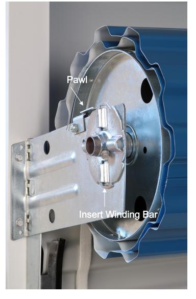
removed, placed the curtain in a fully open position. Insert the winding bar into the tensioner and apply a slight amount of pressure so that you can carefully lift the ratchet pawl. Then, while rotating the tension device in a counterclockwise direction, carefully release the pawl to allow it to lock into the next available groove.
